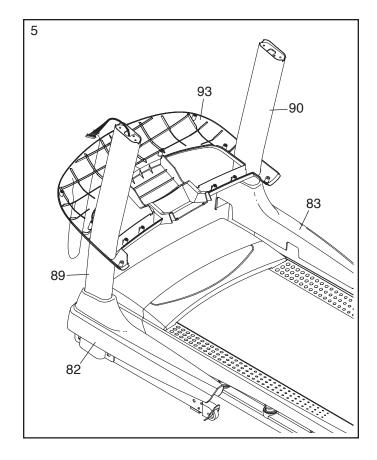
Attach the left handrail assembly (B) to the Left Upright (89) with two 5/16" x 2 1/2" Screws (37) and two 5/16" Star Washers (11). Be careful not to pinch the Upright Wire (81). Start both Screws and then tighten them.
